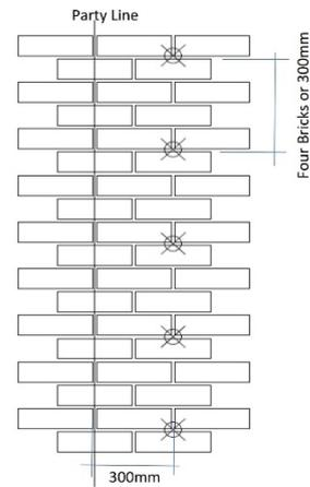
**Diagram 2A** - Typical standard drilling pattern in blockwork detail
