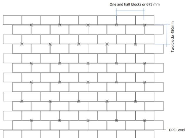
**Diagram 2B** - Typical drilling around windows and doors detail
