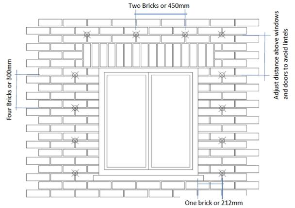
**Diagram 1C** - Typical drilling at roof or eaves level detail
