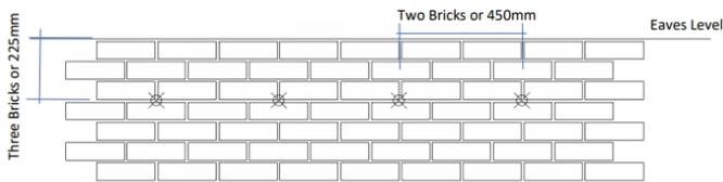
**Diagram 1D** - Typical drilling at a Party Line detail
